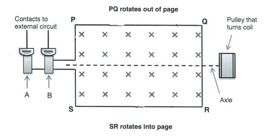
a) Identify components A and B shown on the diagram, explain their function and explain why they are used rather than a commutator.
