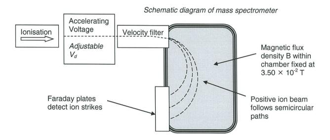
The table below shows the results obtained when the magnetic flux density B in the mass spectrometer was fixed at  $3.50 \times 10^{-2}$  T. Measurements of radius have been expressed with an uncertainty of  $\pm 5\%$  and radius squared with an uncertainty  $\pm 10\%$ .
